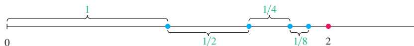
FIGURE 10.8 As the lengths 1, 1/2, 1/4, 1/8, \dots are added one by one, the sum approaches 2.
