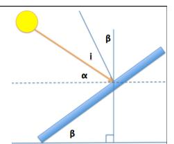
In order to receive the maximum solar radiation, the projection of the normal of the plane must be in the true south. For the collector, i must be zero°
