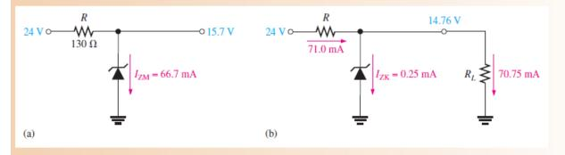
(c) For the minimum load resistance (maximum load current), the zener current is minimum ( $I_{ZK} = 0.25 \text{ mA}$ ) as shown in Figure 3–16(b).
