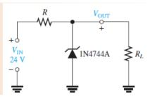
Solution The 1N4744A zener used in the regulator circuit of Figure 3–15 is a 15 V diode. The datasheet in Figure 3–7 gives the following information:
