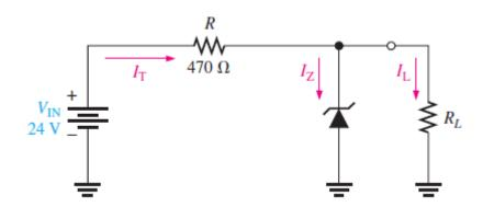
Solution When  $I_L = 0$  A  $(R_L = \infty)$ ,  $I_Z$  is maximum and equal to the total circuit current  $I_T$ .
