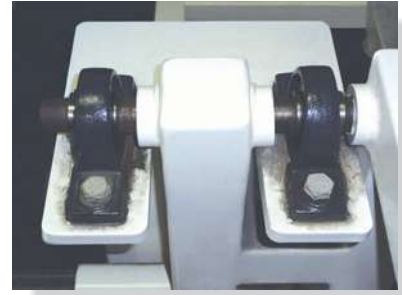
The journal bearings support the ends of the shaft. (5)
