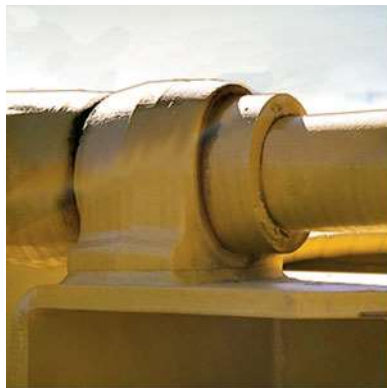
This thrust bearing is used to support the drive shaft on a machine. (7)
