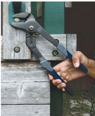
Common tools such as these pliers act as simple machines. Here the applied force on the handles creates a much larger force at the jaws.
