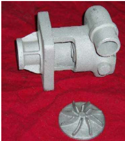
Small water pump for a washing machine. Notice the very simple impeller.
